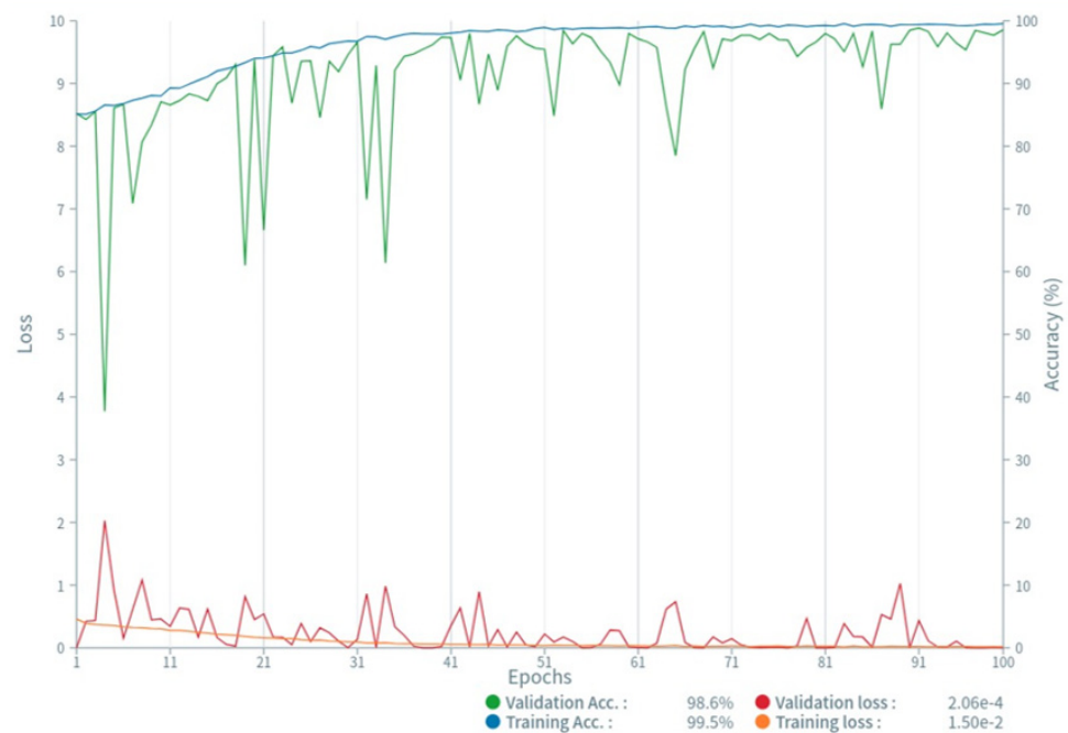
Figure 5. Accuracy and loss of training and validation data. The plots of training loss and validation loss decreased to a stable point, with a small gap between them.
