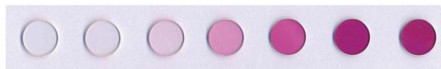
Fig. 1 Coloration of glass A heat treated at 650 °C for different times. The left sample is an untreated reference sample. The other samples were kept at 650 °C for 1, 5, 10, 25, 50, and 100 h (from the left to the right).
