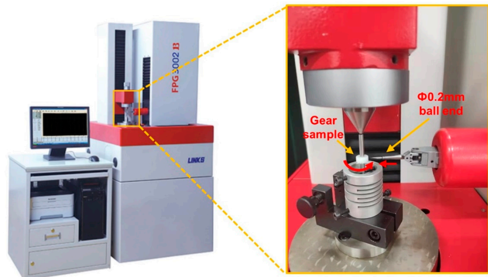
Figure 6. FPG 3002B small-module gear measuring machine and clamping method of small-module gear.
