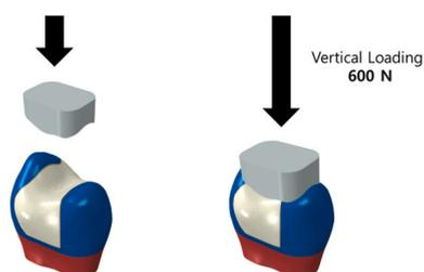
Fig. 3. Illustration of the tooth and food bolus: simulation of 600 N occlusal loading.
