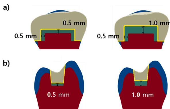
**Fig. 2.** Model design of the thin (left) and thick (right) base material. (a) mesio-distal cross-sectional view, and (b) bucco-lingual cross-sectional view.
