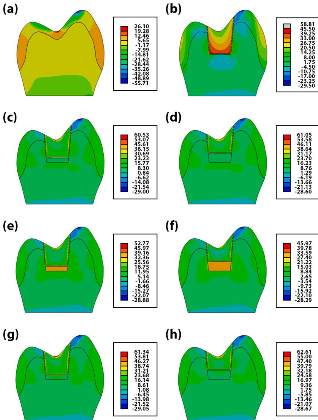
**Fig. 5.** Stress distribution after the shrinkage effect and 600 N vertical loading in the bucco-lingual cross-sectional view. (a) ST, (b) CR, (c) CR-GIC-tk, (d) CR-GIC-tk, (e) CR-LR-tk, (f) CR-LR-tk, (g) CR-TS-tk, and (h) CR-TS-tk.
