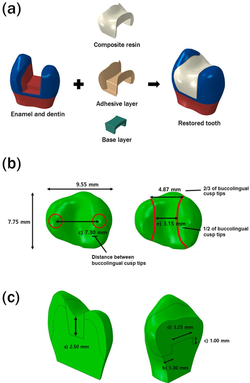
**Fig. 1.** Illustration of the study model design. (a) dentin and enamel, (b) composite resin, (c) adhesive layer, (d) intermediate base, and (e) restored tooth.
