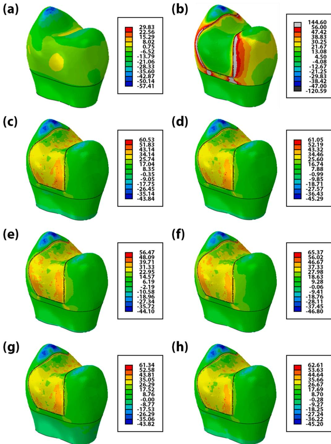
**Fig. 4.** Stress distribution after the shrinkage effect and 600 N vertical loading in the outer view. (a) ST, (b) CR, (c) CR-GIC-tn, (d) CR-GIC-tk, (e) CR-LR-tn, (f) CR-LR-tk, (g) CR-TS-tn, and (h) CR-TS-tk.
