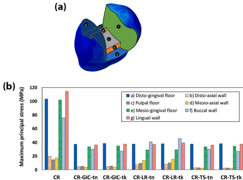
Fig. 6. (A) Labels of each tooth-restoration interface, (b) Comparison in Maximum principal stresses (MPa) on each surface.
