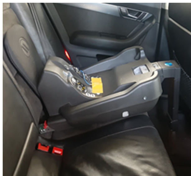
Figure 4. Mounting the acceleration sensor on the Isofix base.
