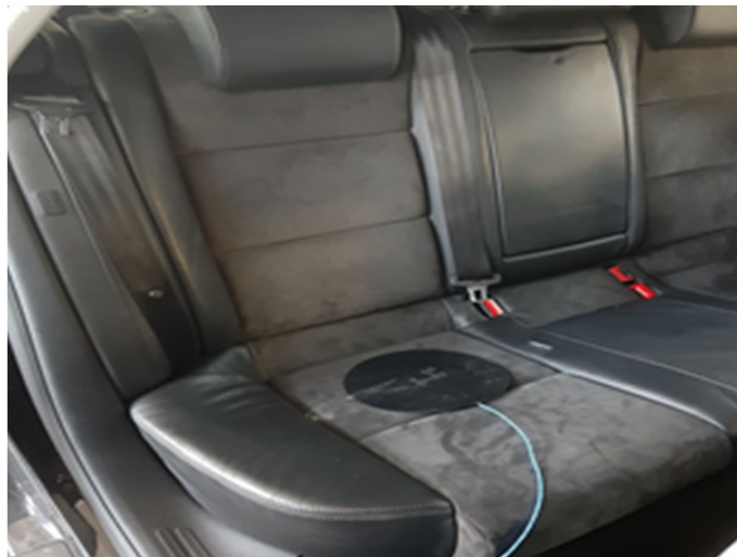
Figure 6. Fixing the acceleration sensor to the rear seat.
