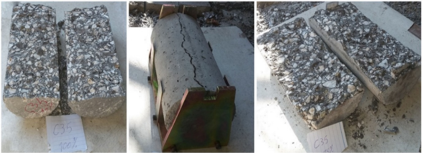
Figure 11. The dominant failure mode for cylindrical samples.
