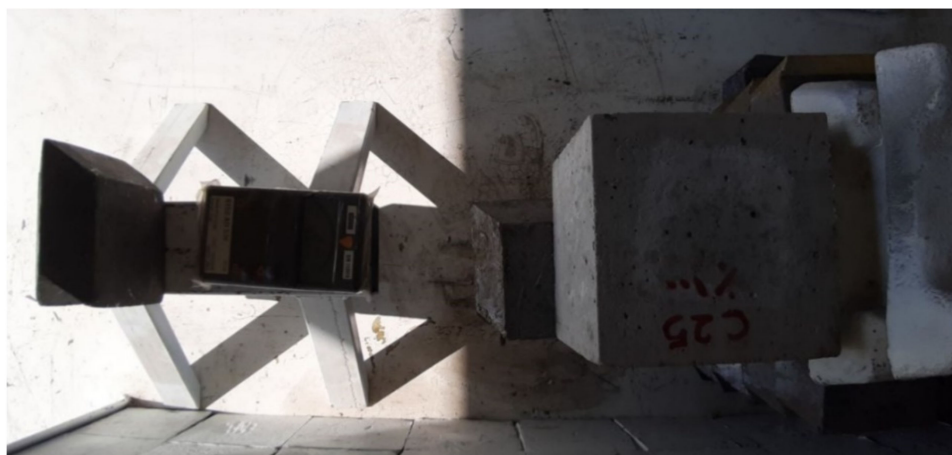
Figure 7. Gamma-ray transmission measurement test setup in the lab.
