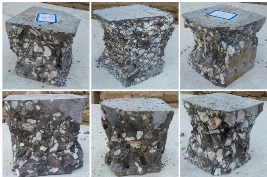
Figure 10. The dominant failure mode for cubic samples.
