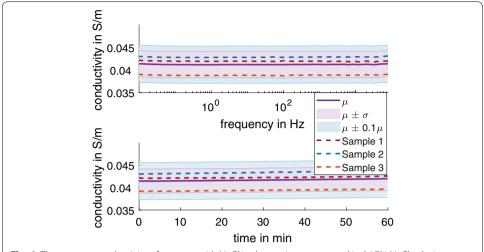
**Fig. 6** The average conductivity of gypsum with NaCl in the casting compound in 0.17% NaCl solution at 25 °C for the (top) extended frequency range of 0.01 Hz to 100 kHz and (bottom) extended duration of 60 min at 10 Hz. The dashed line shows the data for each sample as color-coded. The shaded regions show  $\mu\pm\sigma$  (purple) and  $\mu\pm0.05\mu$  (blue) for comparison
