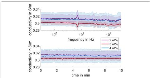
**Fig. 2** The average conductivity of 2 wt% (n = 3), 3 wt% (n = 3), and 4 wt% (n = 3) agar in 0.17% NaCl solution adjusted to 25 °C for (top) frequencies of 0.1 Hz to 100 kHz and (bottom) 1 Hz for 10 min. Three series of measurements were done for each sample with 30 min in between. The shaded regions show  $\mu \pm \sigma$
