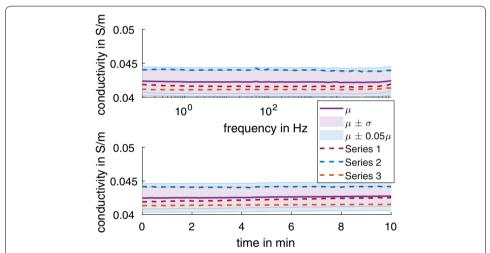
**Fig. 5** The average conductivity of the gypsum sample with NaCl in the casting compound from three series of measurements (color-coded dashed lines) in 0.17% NaCl solution adjusted to 25 °C for (top) frequencies of 0.1 Hz to 100 kHz and (bottom) 1 Hz for 10 min. The shaded regions show  $\mu\pm\sigma$  (purple) and  $\mu\pm0.05\mu$  (blue) for comparison
