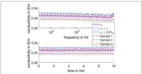
**Fig. 1** The average conductivity data (n = 3) at 25 °C of 0.17% NaCl solution (top) for 0.1 Hz – 100 kHz and (bottom) at 1 Hz for 10 min. The dashed line shows the average for each sample taken over three series of measurements taken with 30 min in between. The shaded regions show  $\mu \pm \sigma$  (purple) and  $\mu \pm 0.01 \mu$  (blue) for comparison
