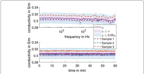
**Fig. 3** The average conductivity of 2 wt% agar in 0.17% NaCl solution adjusted to 25 °C for the (top) extended frequency range of 0.01 Hz to 100 kHz and (bottom) extended duration of 60 min at 10 Hz. The dashed line shows the data for each sample as color-coded. The shaded regions show  $\mu\pm\sigma$  (purple) and  $\mu\pm0.05\mu$  (blue) for comparison
