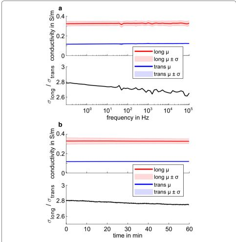
**Fig. 7** The (top) average conductivity and (bottom) anisotropy ratio of reed sticks in 0.17% NaCl solution at 25 °C for **a** frequencies of 0.1 Hz to 100 kHz and **b** duration of 60 min at 10 Hz. The shaded regions show  $\mu\pm\sigma$  for data in longitudinal (red) and transverse (blue) direction
