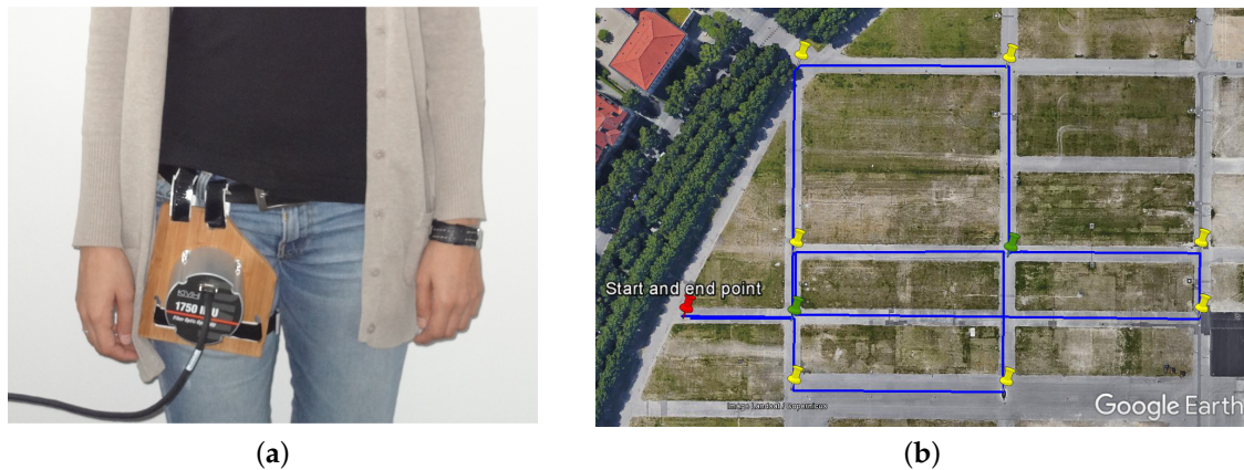
Figure 8. (a) IMU DSP-1750 test set up. (b) trajectory of the experiment represented with a blue line. The pins highlight the corners described during the walk.
