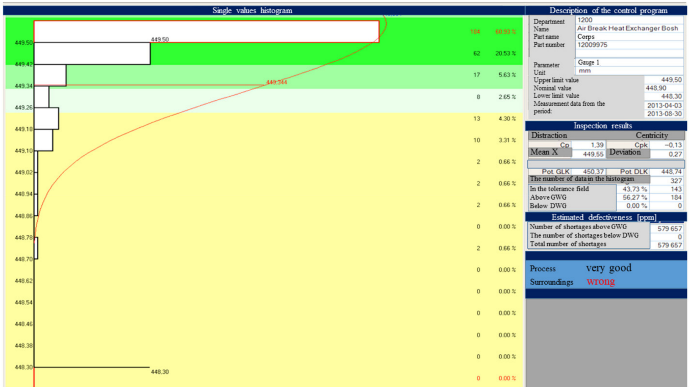
Figure 26. Histogram showing an anomaly in the process.
