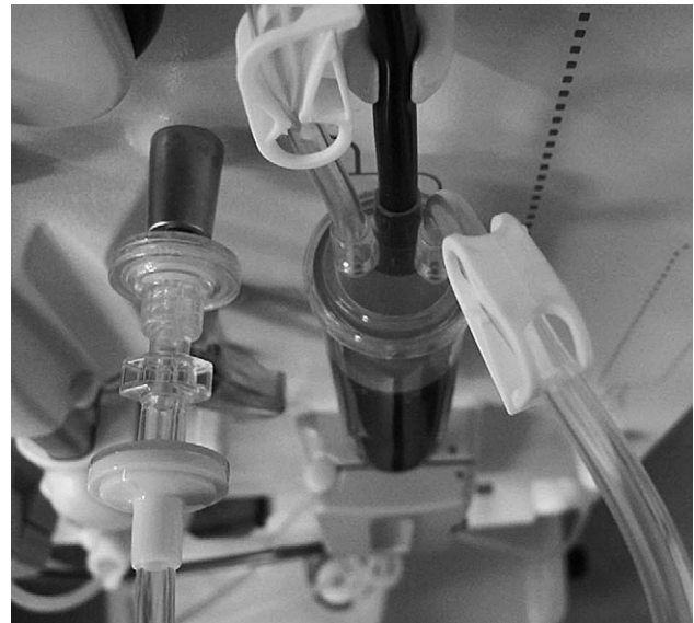
Fig. 1. Double transducer protectors on the venous pressure monitoring line.
