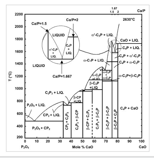
**Figure 3.** Phase diagram of the system CaO-P<sub>2</sub>O<sub>5</sub> (C = CaO, p = P<sub>2</sub>O<sub>5</sub>) at elevated temperatures. Here:  $C_{7}P_{5}$  means 7CaO-5P<sub>2</sub>O<sub>5</sub>; other abbreviations should be written out in the same manner. Reprinted from references 110 and 111 with permission.
