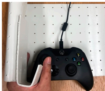
Figure 12. Use of a restraining device to reproduce the insufficient input scenario.
