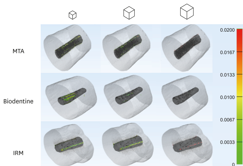
Figure 3. Three-dimensional models representing the interface gaps/voids of the MTA, Biodentine, and IRM cements at 5 (small cube representing the smaller voxel size), 10 (medium cube representing the medium voxel size), and 20 \mu\text{m} (large cube representing the larger voxel size). The color map shows the thickness (mm) of the voids. MTA, mineral trioxide aggregate; IRM, intermediate restorative material.
