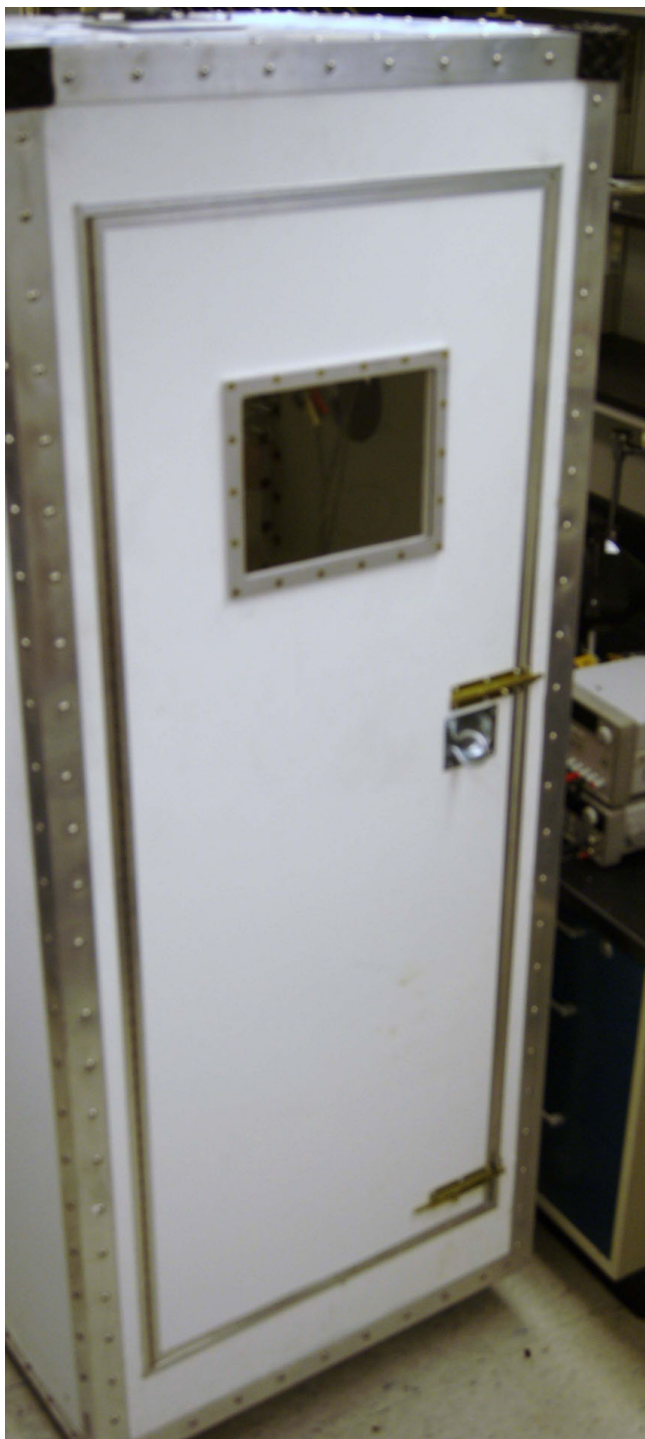
Figure 4 Photo of the Self-cleaning Unit for the Decontamination of Small instruments.
