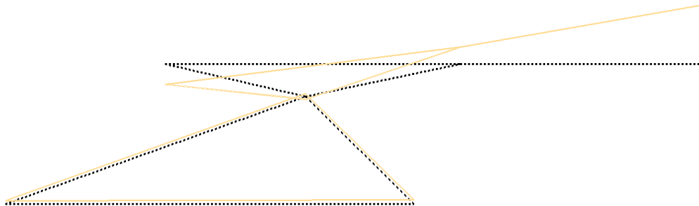
Figure 6. Modal shape of the in-plane torsional mode for the steel specimen case.
