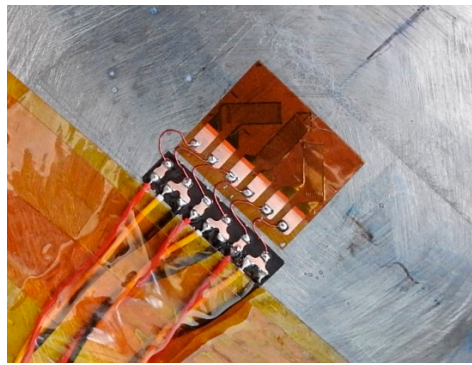
Figure 11. Foil strain gauge with adjacent solder tabs.
