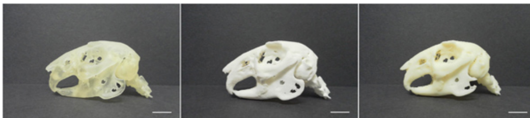
Figure 2. 3D printed models of an ex vivo rabbit skull data set. The objects displayed were printed using a ProJet HD 3000 (left), Shapeways Inc. (Center) and a Makerbot Replicator (right). The scale bar denotes 1 cm.
