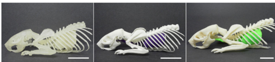
Figure 1. 3D printed models of the lungs and skeletal features of a rat X-ray CT data set. Objects were printed using a ProJet HD 3000 (left), Shapeways Inc. (Center) or a Makerbot Replicator (right). The scale bar denotes 2 cm. Note that the scale bar in panel C is smaller than that of A and B, which reflects that in some cases the Makerbot must print an enlarged object in order to output sufficient detail.
