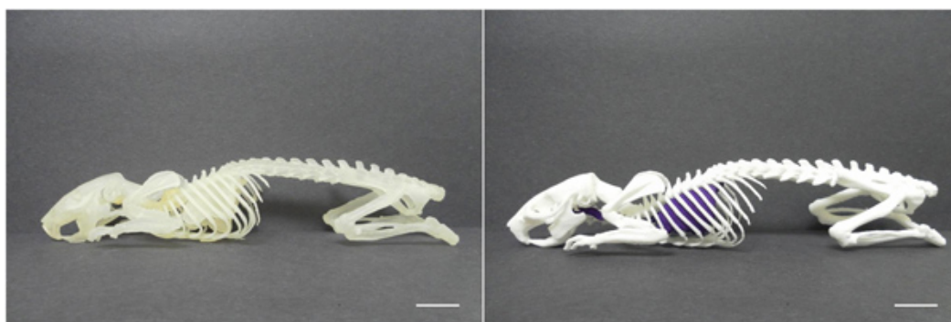
Figure 3. 3D printed models of a full rat X-ray CT data set. Objects were printed using a ProJet HD 3000 (left), and Shapeways Inc. (right). The scale bar denotes 1 cm.
