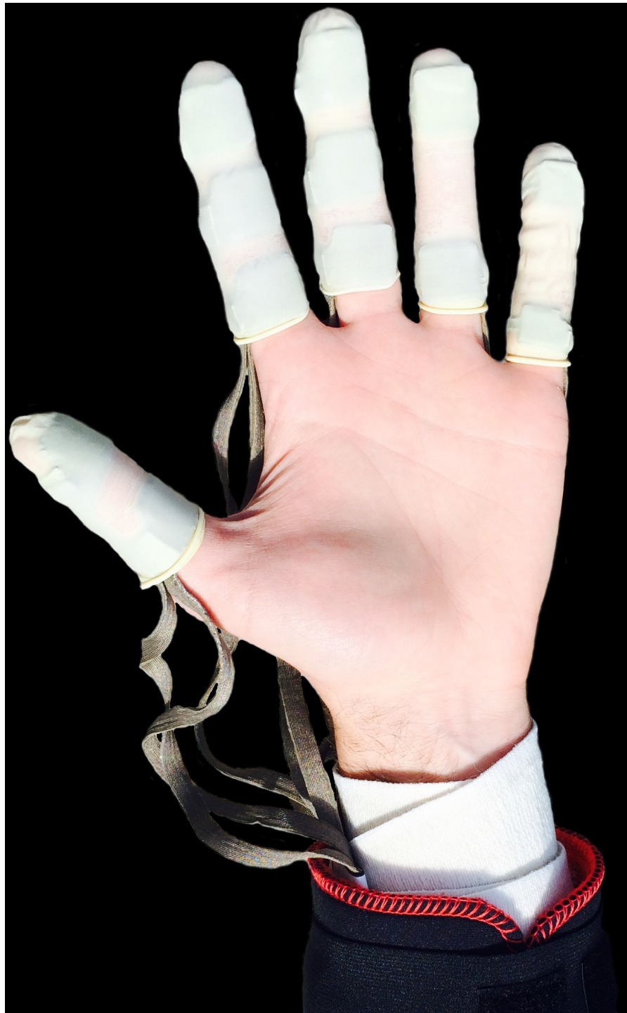
Figure 5 The Novel Pliance ® pressure system attached to the hand of knapper #1. Note the 12 sensors secured underneath the finger cots. Source: A Key.
