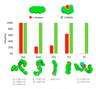
**Figure 6.** Representation of predicted solubilities of some lipids in *n*-hexane and 2-MeOx and their corresponding sigma surfaces, from [32,56]. TAG = Triglycerides, DAG = Diglycerides, FFA = Free fatty acid, ST1 =  $\beta$ -sitosterol, PC = Phosphatidylcholine. Rating: 0–20% bad solvent; 20–60% average solvent; 60–100% good solvent.
