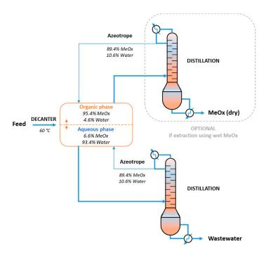
Figure 8. Dry 2-MeOx recovery process.
