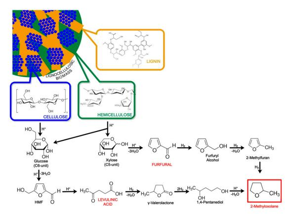
Figure 1. Production of 2-methyloxolane (2-MeOx).
