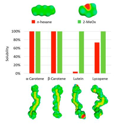
**Figure 5.** Representation of predicted solubilities of some carotenoids in *n*-hexane and 2-MeOx from [46] and their corresponding sigma surfaces, given by COSMO-RS. Rating: 0–20% bad solvent; 20–60% average solvent; 60–100% good solvent.
