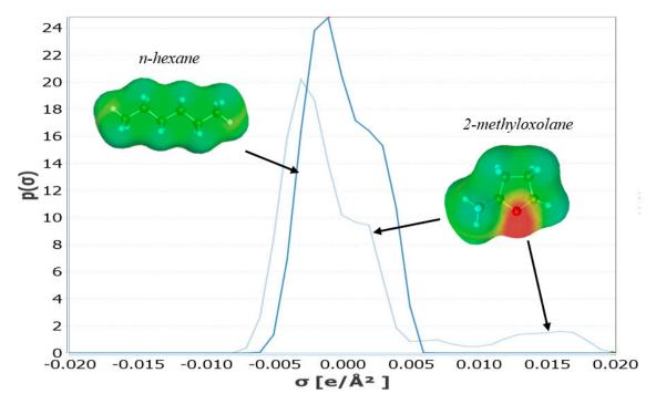
**Figure 3.** σ-surfaces and σ-profiles of 2-MeOx vs. n-hexane. Yellow/Red: molecule charge density <0, Green: molecule charge density = 0 [36].
