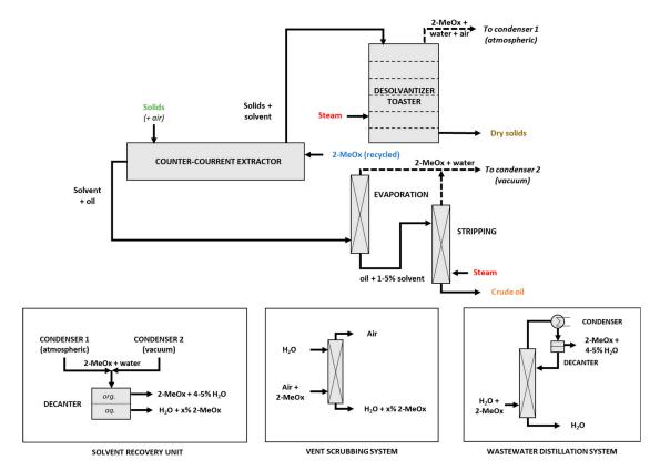
Figure 11. Simplified process diagram of the ENAT International facility (Salamenca, Mexico).
