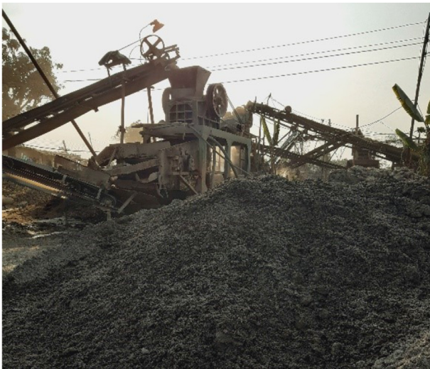
Figure 1. Stone dust as by-product of stone crushing.
