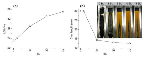
**Figure 14.** Results from LOI (a) and flame spread tests (b) for untreated and LbL-treated silk fabrics. Reprinted with permission from [43]. Copyright 2019, Elsevier.
