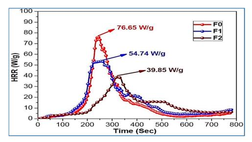
**Figure 6.** Heat release Rate (HRR) vs. time curves for the different systems investigated: F0 (without silica nanoparticles), F1 (with  $2\% \ w/w$  silica nanoparticles) and F2 (with  $4\% \ w/w$  silica nanoparticles). Reprinted with permission from [37]. Copyright 2020, Elsevier.
