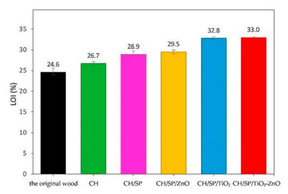
**Figure 32.** Limiting Oxygen Index values for uncoated and LbL-treated wood. CH: Chitosan-coated (green); CH/SP: chitosan sodium phytate-coated (purple); CH/SP/nano-ZnO: chitosan/sodium phytate/nano-ZnO-coated (yellow); CH/SP/nano-TiO<sub>2</sub>: chitosan/sodium phytate/nano-TiO<sub>2</sub>-coated (blue); CH/SP/nano-TiO<sub>2</sub>-ZnO: chitosan/sodium phytate/nano-TiO<sub>2</sub>-ZnO-coated. Reprinted from [57] under CC BY 4.0 license.
