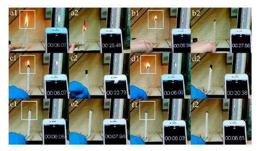
**Figure 33.** Propensity for flame burning of wood and the coated samples: (a1,a2) original wood; (b1,b2) chitosan-coated sample; (c1,c2) chitosan sodium phytate-coated sample; (d1,d2) chitosan/sodium phytate/nano-ZnO-coated sample; (e1,e2) chitosan/sodium phytate/nano-TiO<sub>2</sub>-coated sample; (f1,f2) chitosan/sodium phytate/nano-TiO<sub>2</sub>-ZnO-coated sample. Reprinted from [57] under CC BY 4.0 license.
