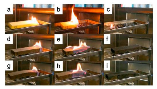
**Figure 29.** Pictures of horizontal flame spread tests of untreated polyurethane foam (**a–c**), foam coated with 3 chitosan/graphene oxide bi-layers (**d–f**) and foam coated with 6 chitosan/graphene oxide bi-layers (**g–i**). First column, right after ignition; second column, 15 s after ignition; third column, during flame out. Reprinted with permission from [56]. Copyright 2018, Elsevier.
