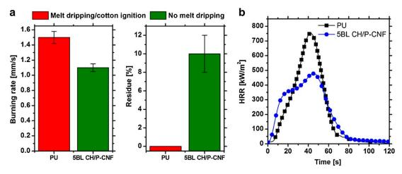
**Figure 28.** Burning rates and final residues evaluated by flame spread tests performed in horizontal configuration (**a**) and Heat Release Rate (HRR) plots as a function of time measured by cone calorimetry tests (**b**). PU: untreated polyurethane foam; 5 BL CH/P-CNF: foam treated with 5 bi-layers of chitosan and phosphorylated cellulose nanofibrils. Reprinted with permission from [55]. Copyright 2018, Elsevier.
