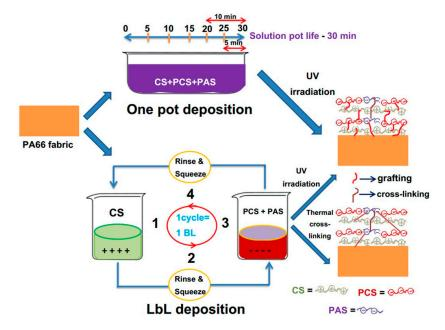
**Figure 16.** Scheme of the LbL vs. "one pot" deposition on polyamide 66 fabrics. CS = chitosan, PCS = phosphorylated chitosan, PAS = polyacrylate sodium, PA66 = polyamide 66. Reprinted with permission from [47]. Copyright 2020, Elsevier.
