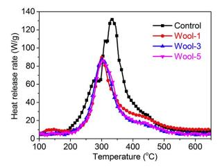
**Figure 23.** Heat Release Rate vs. temperature for untreated wool ("Control") and for the fabric treated with the polyelectrolyte complex with different deposit times. Reprinted with permission from [52]. Copyright 2019, Elsevier.
