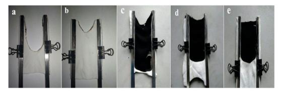
**Figure 20.** Digital images of uncoated and coated polyester fabrics after Limiting Oxygen Index testing. (a) uncoated polyester, (b) LbL-treated polyester—1 bi-layer, (c) LbL-treated polyester—5 bi-layers, (d) LbL-treated polyester—10 bi-layers and (e) LbL-treated polyester—20 bi-layers. Reprinted with permission from [50]. Copyright 2019, Elsevier.
