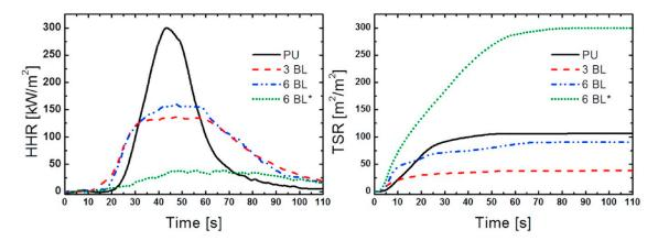
**Figure 30.** Heat Release Rate (a) and Total Smoke Release (TSR) curves of untreated polyurethane foam (PU) and of foams coated with 3 ("3BL") and 6 ("6BL") chitosan/graphene oxide bi-layers. 6BL\* indicates non-igniting samples. Reprinted with permission from [56]. Copyright 2018, Elsevier.
