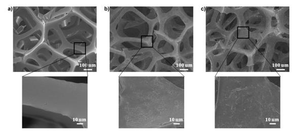
**Figure 25.** Scanning Electron Microscopy (SEM) images of (a) uncoated polyurethane foam; (b,c) foam coated with 10 bi-layers of chitosan/sodium montmorillonite at pH = 3 (panel (b)); foam coated with 10 bi-layers of chitosan/sodium montmorillonite at pH = 6 (panel (c)). Reprinted with permission from [53]. Copyright 2012, American Chemical Society.
