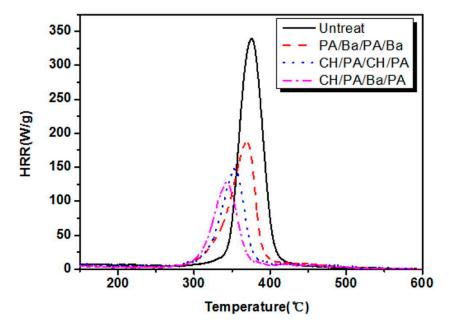
**Figure 13.** Results from pyrolysis-combustion flow calorimetry tests. PA/Ba/PA/Ba: quad-layer made of phytic acid/Ba<sup>2+</sup>/phytic acid/Ba<sup>2+</sup>; CH/PA/CH/PA: quad-layer made of chitosan/phytic acid/chitosan/phytic acid/CH/PA/Ba/PA: quad-layer made of chitosan/phytic acid/Ba<sup>2+</sup>/phytic acid. Reprinted with permission from [42]. Copyright 2019, Elsevier.
