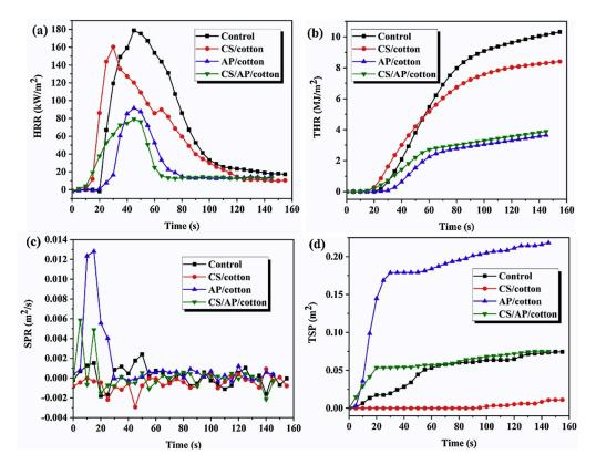
**Figure 19.** Results from cone calorimetry tests for untreated and treated cotton fabrics. Heat Release Rate—HRR (a), Total Heat Release—THR (b), Smoke Production Rate—SPR (c) and Total Smoke Production—TSP (d) curves. Reprinted with permission from [49]. Copyright 2020, Elsevier.
