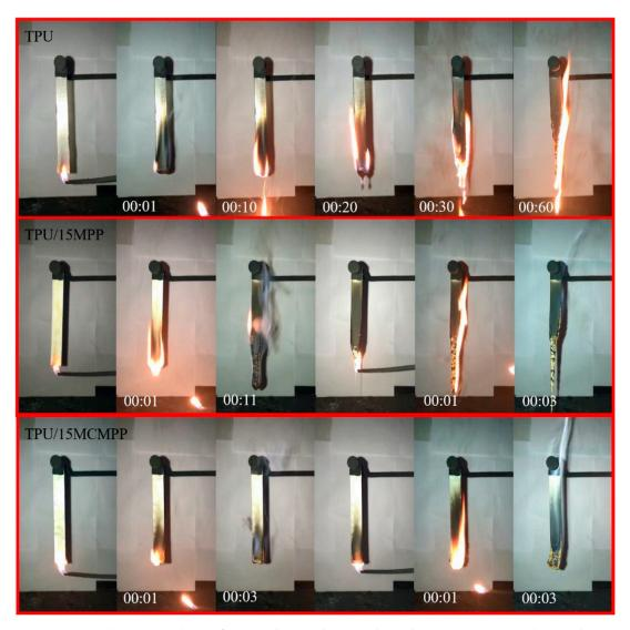
**Figure 4.** Video screenshots of TPU (thermoplastic polyurethane), TPU/MPP (thermoplastic polyurethane containing 15 wt. % of melamine polyphosphate) and TPU/MCMPP (thermoplastic polyurethane containing 15 wt. % of melamine polyphosphate microencapsulated by toluene disocyanate crosslinked carboxymethyl chitosan) composites during UL-94 testing. Reprinted with permission from [32]. Copyright 2019, Elsevier.
