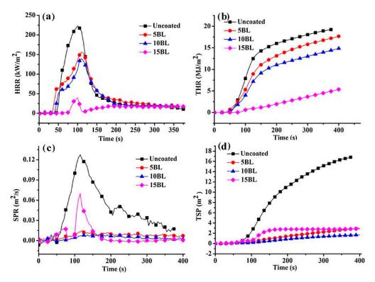
**Figure 10.** Results from cone calorimetry tests for untreated and LbL-treated cotton fabrics. Heat Release Rate—HRR (a), Total Heat Release—THR (b), Smoke Production Rate—SPR (c) and Total Smoke Production—TSP (d) curves. Reprinted with permission from [40]. Copyright 2018, Elsevier.
