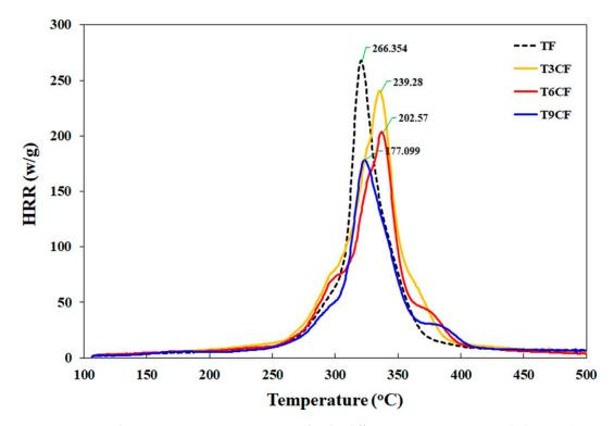
**Figure 5.** Heat Release Rate (HRR) vs. time curves for the different systems investigated: thermoplastic starch–flax fabric (TF), thermoplastic starch–chitosan–flax fabric (TXCF, where X indicates the weight % of chitosan). Reprinted with permission from [36]. Copyright 2018, Elsevier.
