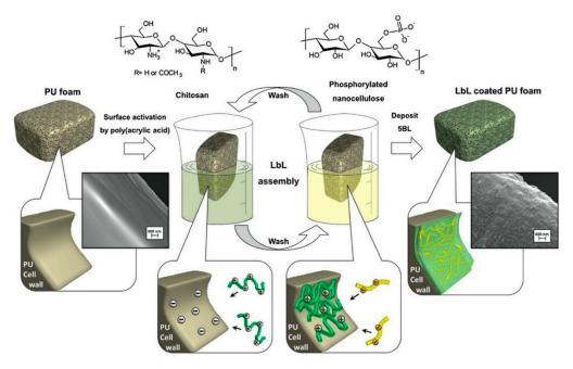
**Figure 27.** Schematic representation of the LbL process. Polyurethane foams were pre-activated by poly(acrylic acid) and then alternatively dipped in the chitosan (positive) and phosphorylated cellulose nanofibrils (negative) baths. The process was repeated 5 times in order to deposit 5 bi-layers. Reprinted with permission from [55]. Copyright 2018, Elsevier.
