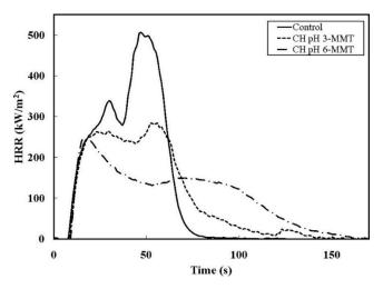
**Figure 26.** Heat-Release Rate (HRR) as a function of time during cone calorimeter testing for control (uncoated polyurethane foam) and for the foams coated with 10 bi-layers of chitosan/sodium montmorillonite at pH = 3 (CH pH 3-MMT) and at pH = 6 (CH pH 6-MMT). Reprinted with permission from [53]. Copyright 2012, American Chemical Society.
