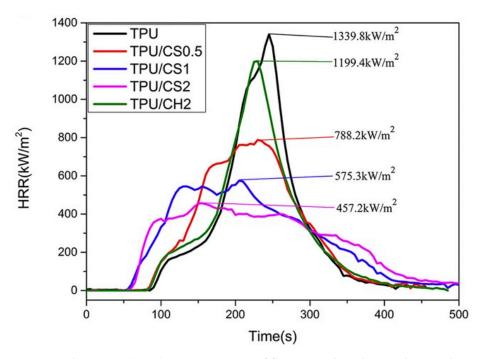
**Figure 7.** Heat Release Rate (HRR) vs. time curves of flame retardant thermoplastic polyurethane elastomer (TPU) composites. CH, chitin, CS, chitosan. Reprinted with permission from [38]. Copyright 2020, Wiley.
