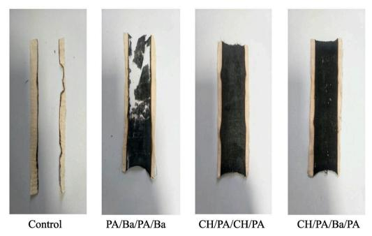
**Figure 12.** Residues at the end of the flame spread tests performed in a horizontal configuration. PA/Ba/PA/Ba: quad-layer made of phytic acid/Ba<sup>2+</sup>/phytic acid/Ba<sup>2+</sup>; CH/PA/CH/PA: quad-layer made of chitosan/phytic acid/chitosan/phytic acid; CH/PA/Ba/PA: quad-layer made of chitosan/phytic acid/Ba<sup>2+</sup>/phytic acid. Reprinted with permission from [42]. Copyright 2019, Elsevier.
