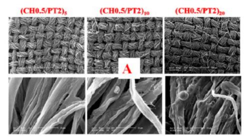
**Figure 9.** SEM images, at different magnification, of the residues of the LbL-treated fabrics after vertical flame spread tests. 5, 10 and 20 correspond to the number of deposited bi-layers. CH = chitosan; PT = phosphorylated chitin; 0.5 and 2 are the wt. % concentrations of the biomacromolecules in the dipping baths. Reprinted with permission from [39]. Copyright 2015, Elsevier.
