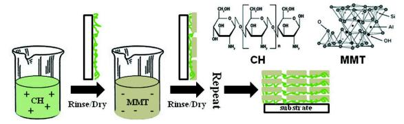
**Figure 24.** Schematic representation of Layer-by-Layer (LbL) assembly with chitosan (CH) and sodium montmorillonite clay (MMT). This process is repeated until the desired number of bilayers is deposited. Reprinted with permission from [53]. Copyright 2012, American Chemical Society.
