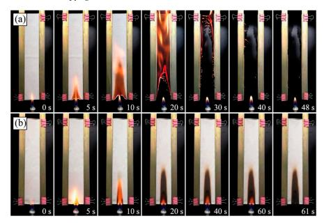
**Figure 21.** Vertical burning test processes of (a) untreated cotton fabric and (b) cotton fabric coated with the system containing 50 wt. % of modified montmorillonite in the carboxymethyl chitosan/montmorillonite treating bath, with four repetitions of the dip-coating process. Reprinted with permission from [51]. Copyright 2019, Elsevier.
