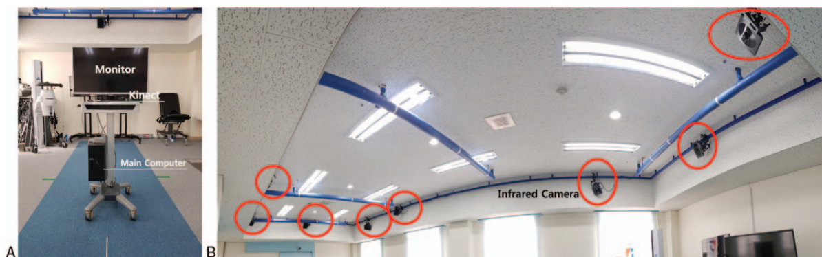
Figure 1. POM-Checker and motion capture system. POM-Checker consists of main computer, monitor, and Kinect. 3D motion capture system has 8 infrared cameras. (A) It is anterior view of POM-Checker. (B) Panorama view of BTS SMART DX-400 at GJWMC. This motion capture system has 8 infrared cameras. Seven cameras are only shown in the picture.
