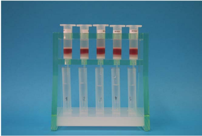
Figure 1. Column rack with mounted columns and trypanosomes being eluted from the blood in the collector tubes. doi:10.1371/journal.pntd.0000471.g001
