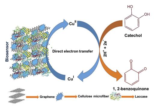
Figure 8. Schematic representation for the electrochemical redox behavior of laccase and electro-oxidation mechanism of CC by the as-prepared laccase biosensor.
