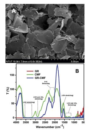
**Figure 3.** (**A**) High resolution SEM image of SPCE modified GR-CMF composite. (**B**) FTIR spectra of CMF (green line), GR (red line) and GR-CMF composite (blue line).
