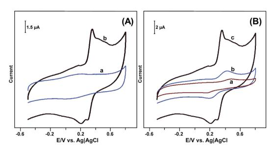
**Figure 7.** (A) Cyclic voltammetric response obtained for GR-CMF/laccase modified SPCE in the absence (a) and presence (b) of 50  $\mu$ M CC in pH 5 at a scan rate of 100 mV/s. (B) At similar conditions, the cyclic voltammetry response of CMF (a), GR-CMF (b) and GR-CMF/laccase (c) modified SPCEs towards 50  $\mu$ M CC.
