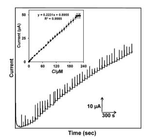
Figure 9. Amperometric *i-t* response of the GR-CMF/laccase modified SPCE for different concentration additions (0.2 to 224.7  $\mu$ M) of CC into the constantly stirred 0.1 M sodium phosphate buffer pH 5.0; Working potential = +0.4 V. Inset is the linear plot for the amperometric current response vs. [CC].
