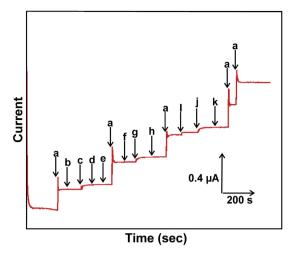
**Figure 10.** Amperometric *i*-*t* response of the biosensor for the addition of  $1 \mu M CC$  (a) and  $50 \mu M$  additions of hydroquinone (b), dopamine (c), resorcinol (d), phenol (e), 2-amino phenol (f), pyrogallol (g), caffeic acid (h), gallic acid (i), catechin (j) and phloroglucinol (k) into the constantly stirred 0.1 M sodium phosphate buffer pH 5.0.
