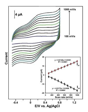
**Figure 5.** Cyclic voltammetry response obtained for laccase immobilized on GR-CMF modified SPCE in pH 5.0 at different scan rates from 100 to 1000 mV/s. Inset is the linear plot for anodic and cathodic peak current of laccase redox couple vs. scan rate.
