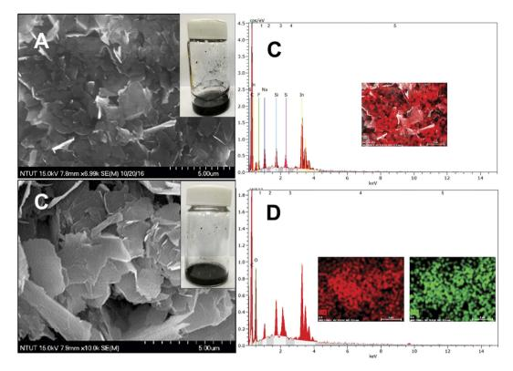
**Figure 2.** High resolution SEM images of GR (**A**) and GR-CMF composite (**C**). Optical images of GR dispersion in DMF (inset of A) and CMF (inset of C). The EDS and elemental mapping of GR (**B**) and GR-CMF composite (**D**).
