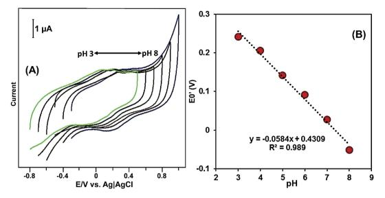
**Figure 6.** (**A**) Cyclic voltammetric behavior of GR-CMF/laccase modified SPCE in different pH (pH 3–8) at a scan rate of 100 mV/s. (**B**) Linear plot for formal potential of laccase redox couple vs. pH.
