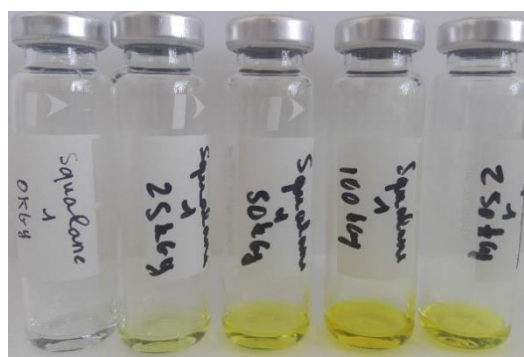
Figure 3. Non-irradiated and \gamma -irradiated 2,6-di-tert-butyl-p-cresol in polymer matrix simulating (left to right: 0, 25, 50, 100, and 250 kGy).
