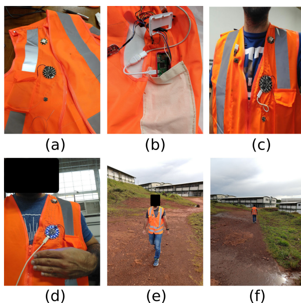
Figure 6. Wearable prototype for surface mining environments: (a) prototype during its development. (b) Prototype internal pocket holding Raspberry Pi Zero W platform. (c,d) In-lab development tests. (e,f) Prototype deployment, field tests and validation.
