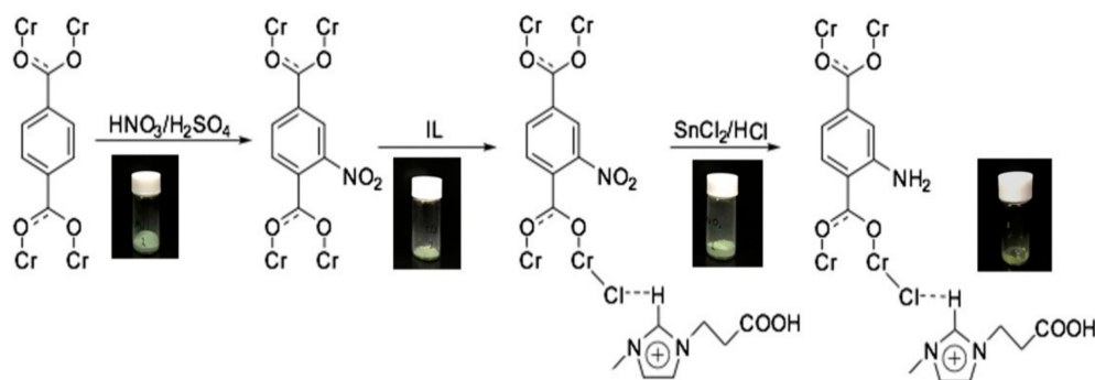
Figure 20. Preparation stages for the synthesis of IL/MIL-101-NH 2 . Reprinted with permission from Ref. [158]. Copyright 2018 Elsevier.
