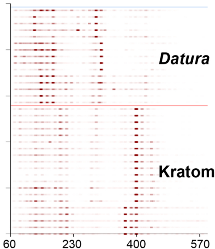
Figure 4. Heat map renderings of the direct analysis in real time-high resolution mass spectrometry spectra of Kratom and Datura plant materials. High intensity peaks are shown in dark red and lower intensity peaks are indicated in lighter shades. Please click here to view a larger version of this figure.
