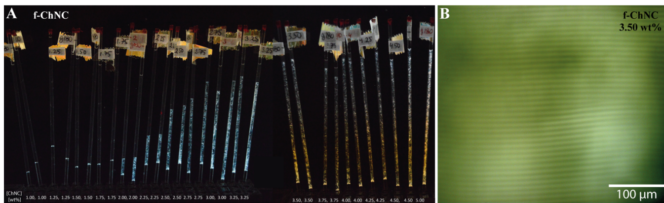
Figure S4. Self-assembly behavior of ChNCs derived from fungi. (A) Photograph of capillaries filled with f-ChNC suspension with increasing concentration. (B) The fingerprint pattern, characteristic for chiral nematic phase, was imaged by polarized optical microscopy for a 3.50 wt% ChNC suspension.
