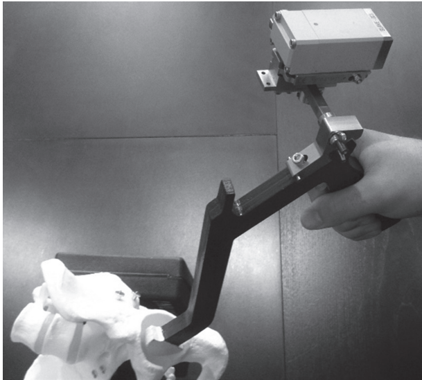
Fig. 2a Dry-bone model showing an example sensor attached to a mock reamer (Image courtesy of InLine Orthopaedics).
