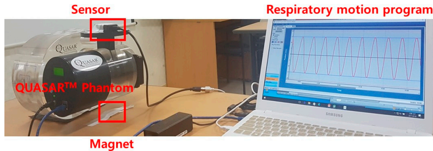
Figure 3. Experimental setup for measuring sensor signals with the QUASAR™ Programmable Respiratory Motion Phantom and respiratory motion program.
