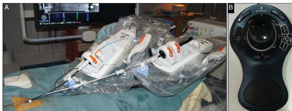
Figure 4 (A) Final setup of the arms of the V-Drive Duo (with V-CAS Deflect and V-Loop) at the sheath insertion site. (B) The V-Drive controller that allows remote manipulation of the ablation catheter, its sheath and of the lasso.
