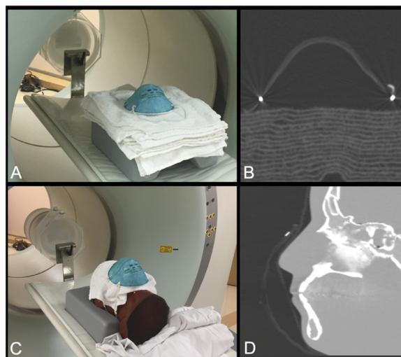
**Figure 1.** CT acquisition of a commercial N95 respirator to aid in generation of a 3D printed mask. Photographs and computed tomography (CT) acquisition images of a commercial N95 respirator in isolation (A, B) and positioned on an anthropomorphic head CT phantom (C, D). (Color version of figure is available online.)
