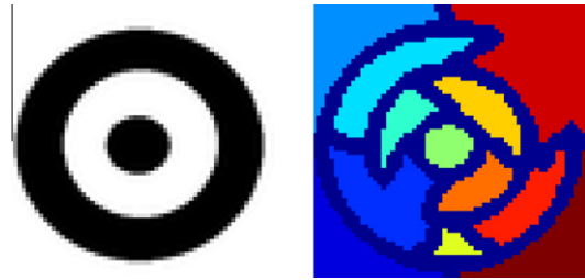
Fig. 2. Illustration of selection regions for a concentric circle example. Left: original image. Right: automatically determined selection regions using quick-shift followed by an erosion. Different colors represent different regions. Dark-blue indicates regions not covered by the selection regions, for which pixels are not controlled by selection regions and can therefore faithfully represent segmentation boundaries. (For interpretation of the references to color in this figure legend, the reader is referred to the web version of this article.)
