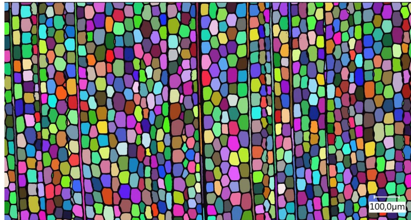
Figure 2. Example of pore lumina detection by microscopic measurements of douglas fir sapwood (earlywood).
