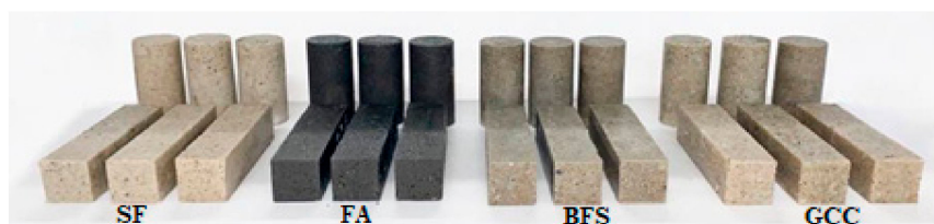
Figure 3. Specimen shape, depending on the type of filler; silica flour (SF), fly ash (FA), blast furnace slag (BFS), and ground calcium carbonate (GCC).
