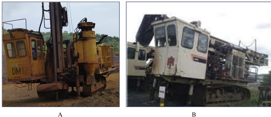
Fig. 1. Study drill machines from two manufacturers. (A) Atlas Copco (Model – IDM30). (B) Ingersoll Rand (Model – DM30E).
