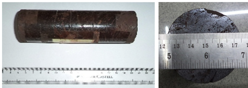
Fig. 3. NX (diameter = 54 mm, length to diameter ratio = 2:1) size of rock core samples for laboratory tests.
