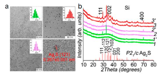
**Figure 1.** Transmission electron microscopy (TEM) images with size histograms of  $Ag_2S$  quantum dots (QDs) deposited on an Si substrate (**a**); X-ray diffraction (XRD) patterns of  $Ag_2S$  QDs with different sizes (1–3), curves with dashed numbers (1'–3') respect to  $Ag_2S$  QDs deposed on Si substrate (**b**).
