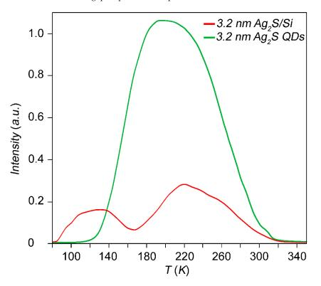
**Figure 6.** Curves of thermoluminescence for Ag<sub>2</sub>S QDs colloidal solutions (top curve) and Ag<sub>2</sub>S QDs deposed on Si substrate (bottom curve) with average size of 3.2 nm.
