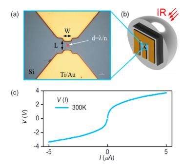
**Figure 4.** (a) An optical image of the inner part of the device; infrared (IR) radiation is focused on the Si surface between the Ti/Au contacts. (b) An image of the device mounted on the Si lens. (c) An IV curve of the Au/Ti/Si/Ti/Au structure; the shape of the IV curve indicates the formation of a spatial charge distribution at the Si/Ti interface.
