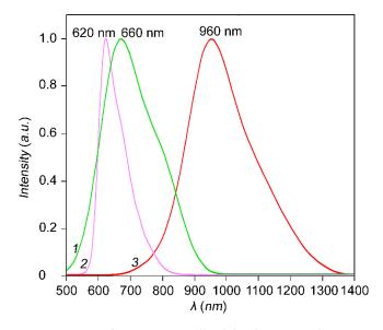
**Figure 3.** Luminescence spectra of  $Ag_2S$  QDs colloidal solutions. The maxima of luminescence bands are at 660 nm, 620 nm, and 950 nm for  $Ag_2S$  QDs with average size of 1.8 nm, 2.0 nm and 3.2 nm respectively.
