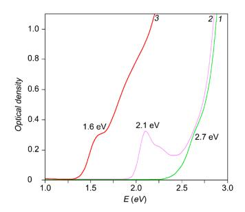
**Figure 2.** Optical absorbance spectra of Ag<sub>2</sub>S QDs colloidal solutions. The curves have characteristic features at of 1.6 eV, 2.1 eV, and 2.7 eV, for solutions with an Ag<sub>2</sub>S QDs average size of 3.2 nm, 2.0 nm, and 1.8 nm, respectively.
