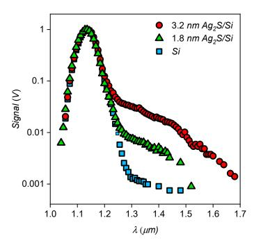
**Figure 5.** Spectral response curves of the uncovered Si and Ag<sub>2</sub>S/Si heterostructures. The comparison of the curves reflects a sub-band gap IR photon absorption in Si.
