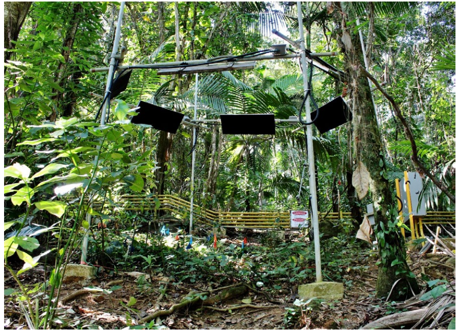
FIGURE 3 Photograph of a heated plot showing the understory vegetation beneath the tree canopy along with six infrared heaters deployed on pipes arranged in a hexagon. The vertical pipes are posts set in concrete footings, two of which are visible in the foreground. The gray control panel is to the right. In the background is the 480 V, 3-phase power line in yellow conduit. (Photo by Mónica Cruz)
