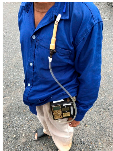
Figure 2. Absorbent tube sampling application.
