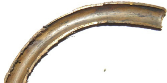
Fig. 17. After test surface of coil inner surface.
