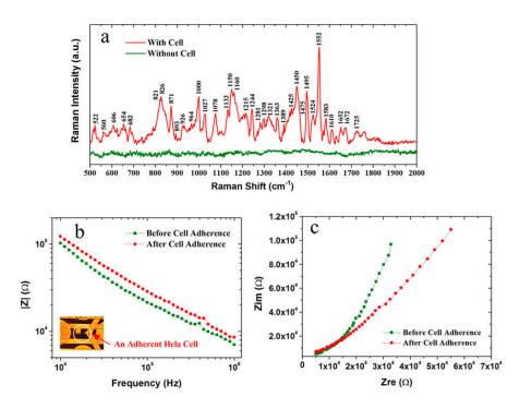
**Figure 11.** Dual-modal detection of a single Hela cell. (a) SERS spectrum of a single Hela cell attaching on the underneath electrode with Au nanostructure; (b) Comparison of cellular impedances before and after its attachment. Inset in (b) is the light microscope image of a single Hela cell adhering on the measuring electrodes; (c) Cole-Cole plots of the impedance measurements. Reproduced with permission from [116]. Copyright Nature Publishing Group, 2015.
