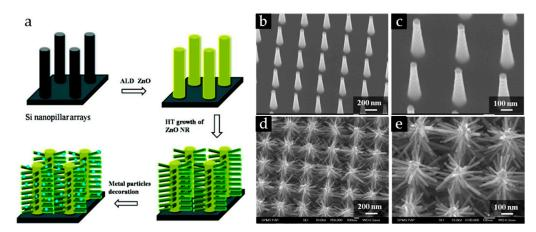
**Figure 7.** (a) Schematic diagram of the fabrication procedures for the three-dimensional ordered Si/ZnO nanotrees decorated by silver nanoparticles; SEM images of the (b) Si nanopillar arrays and the (d) ordered Si/ZnO nanotrees; as well as (c,e) the corresponding magnified SEM images. Reproduced with permission from [105]. Copyright American Chemical Society, 2010. ALD: atomic layer; NR: nanorod; HT: hydrothermal.
