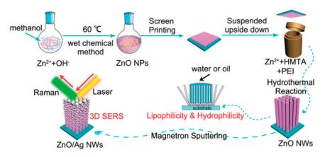
**Figure 6.** Schematic diagram of the preparation process of patterned ZnO nanowire arrays and the three-dimensional ZnO/Ag nanowire surface-enhanced Raman scattering (SERS) substrate. Reproduced with permission from [18]. Copyright The Royal Society of Chemistry, 2016. HMTA: hexamethylenetetramine; NW: nanowire; PEI: ethylene imine polymer.
