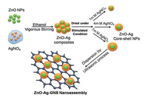
**Figure 13.** Schematic illustration of ZnO–Ag–graphene nanosheet (ZnO–Ag–GNS) nanoassembly synthesized by a wet chemical process. Reproduced with permission from [118]. Copyright The Royal Society of Chemistry, 2016.
