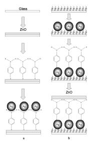
**Figure 9.** Schematic diagram of (a) ZnO/PATP (4-aminothiophenol)/Ag sandwich structure; (b) Ag/PATP/ZnO sandwich structure on glass substrates. Reproduced with permission from [110]. Copyright American Chemical Society, 2008.
