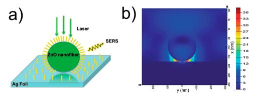
**Figure 10.** (a) Schematic diagram of ZnO nanofibers deposited on the surface of silver foil with probed molecules; (b) The distribution of the electric field for ZnO nanofibers deposited on the surface of silver foil calculated with finite-difference time-domain (FDTD) simulation. Reproduced with permission from [113]. Copyright The Royal Society of Chemistry, 2015.
