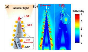
**Figure 12.** Ultrasharp ZnO nanocone arrays hybridized with the plasmonic systems of Au particle on Ag film (a) Schematic showing detection principle of fabricated SERS sensor; (b) Normalized electric field distribution for the ZnO/Ag/PDDA/AuNP NCs. Reproduced with permission from [99]. Copyright American Chemical Society, 2015. PDDA: poly(diallydimethylammonium chloride).
