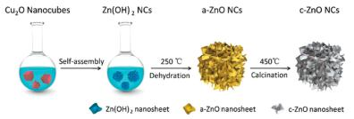
**Figure 2.** Schematic diagram of the synthesis of a- and c-ZnO NCs (amorphous and crystalline ZnO nanocages). Reproduced with permission from [91]. Copyright Wiley-VCH Verlag GmbH & Co. KGaA, Weinheim, 2017.
