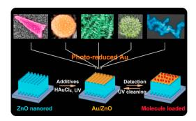
**Figure 8.** The photoinduced Au nanostructures in the form of conical Au, sphere Au, dendritic Au, sea-urchin-like Au, and Au chain from left to right, respectively. Reproduced with permission from [106]. Copyright American Chemical Society, 2016.
