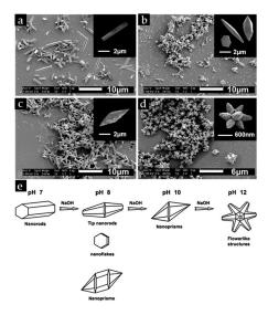
**Figure 3.** SEM images of ZnO deposited on Corning 7059 for a deposition time of 2 h and (**a**) pH 7, (**b**) pH 8, (**c**) pH 10, (**d**) pH 12, and the individual structures are exhibited in the insets of (**a**–**d**); (**e**) shows a schematic map of the morphology of the nanostructures. Reproduced with permission from [43]. Copyright Elsevier B.V., 2007.
