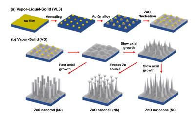
**Figure 5.** Schematic diagram of the growth mechanism of ZnO nanocones, nanorods, and nanonails. (a) Textured ZnO film formed with a vapor–liquid–solid (VLS) mechanism; (b) ZnO nanocones, nanorods, and nanonails grown with the vapor–solid (VS) mechanism. Reproduced with permission from [99]. Copyright American Chemical Society, 2015.
