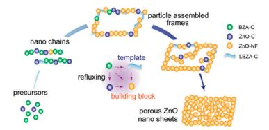
**Figure 4.** Schematic diagram of the composition and morphology evolution of the porous ZnO nanosheets. Reproduced with permission from [94]. Copyright WILEY-VCH Verlag GmbH & Co. KGaA, Weinheim, 2013. BZA-C: basic zinc acetate clusters; LBZA-C: layered basic zinc acetate clusters; ZnO-C: ZnO clusters; ZnO-NP: ZnO nanoparticles.
