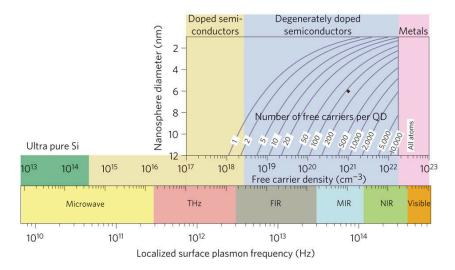
**Figure 1.** Local surface plasmon resonance (LSPR) frequency dependence on the free electron density for semiconductors, and number of free carriers per quantum dot (QD) required for nanosphere diameter ranging from 2 to 12 nm to achieve a free carrier density between  $10^{17}$  and  $10^{23}$  cm<sup>-3</sup>. Reproduced with permission from [65]. Copyright Nature Publishing Group, 2011.
