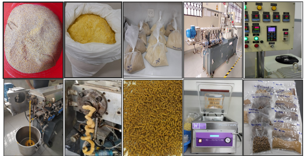
Figure 1. Extruded production workflow. From left to right: At the top—weighing and blending of raw materials; setting up of operation parameters; flour blends feeding and water conditioning. At the bottom—extrusion and cutting of the extrudate into pieces; cooling and storage of the extrudate in bioriented polypropylene bags.
