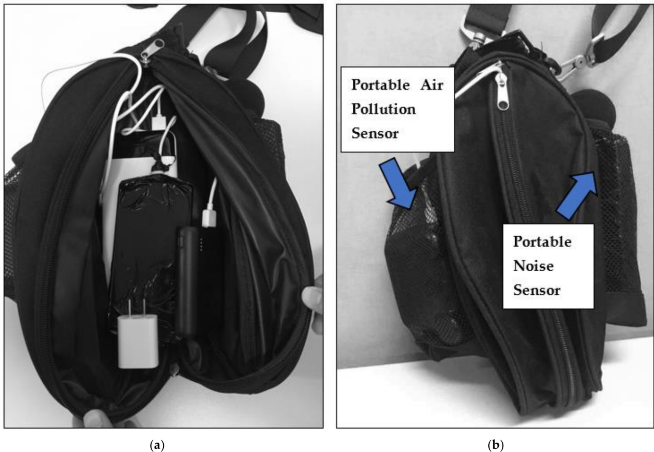
Figure 3. The device bag for the GPS and mobile sensors. (a) The portable devices are packed into a device bag; (b) air pollution sensors and noise sensors are placed in the two external mesh pockets on the two sides of the bag.
