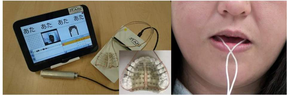
Fig 1. Instrumentation. A tablet-type EPG system and recording system (STARS), and a picture of a participant wearing EPG plate.
