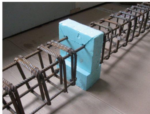
Figure 2. Midspan part of the steel reinforcement skeleton of Series I beams with the foam polystyrene [48].
