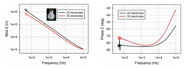
The impedance of the small 3D electrodes in DI water, a 0.1% and 1% NaCl solution is shown in Figure 8. The plotted curves are average values taken from 5 different electrodes on the same chip. The
