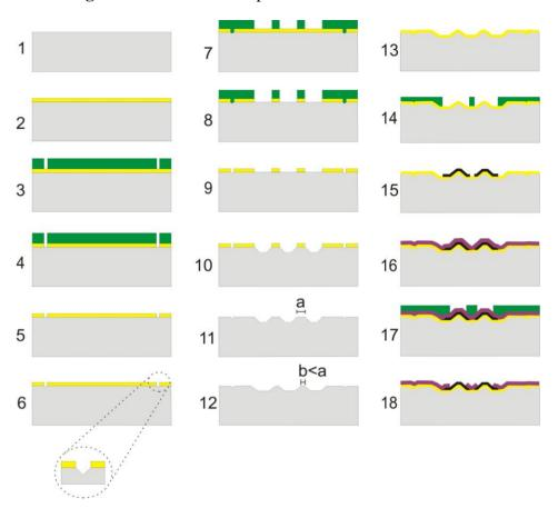
Figure 2. The fabrication process for the small electrodes.
