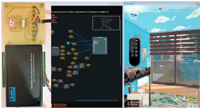
Fig. 5. HOME I/O, CONNECT I/O and 7-segment display
