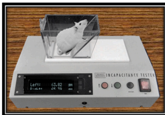
Fig. 4. Measuring weight-bearing capacity of hind paws over the treatment of test samples using in capacitance tester.
