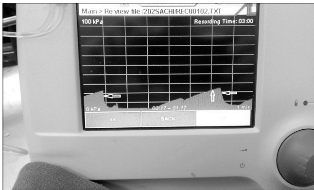
Figure 3: Graphical representation of pressure trace displayed on the monitor screen of the device. Left horizontal arrow showing dip of pressure trace on voluntary release of occlusion (pre-procedural instrument checking) and right horizontal arrow showed sudden fall in pressure trace on localisation of the space sooner the needle pierces ligamentum flavum, while vertical arrow shows gradual rise of pressure as the needle crossing the ligaments
